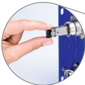
Waterproof optical ports with choice of SFPs
